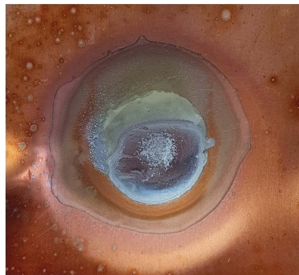
No corrosion: Classification L
